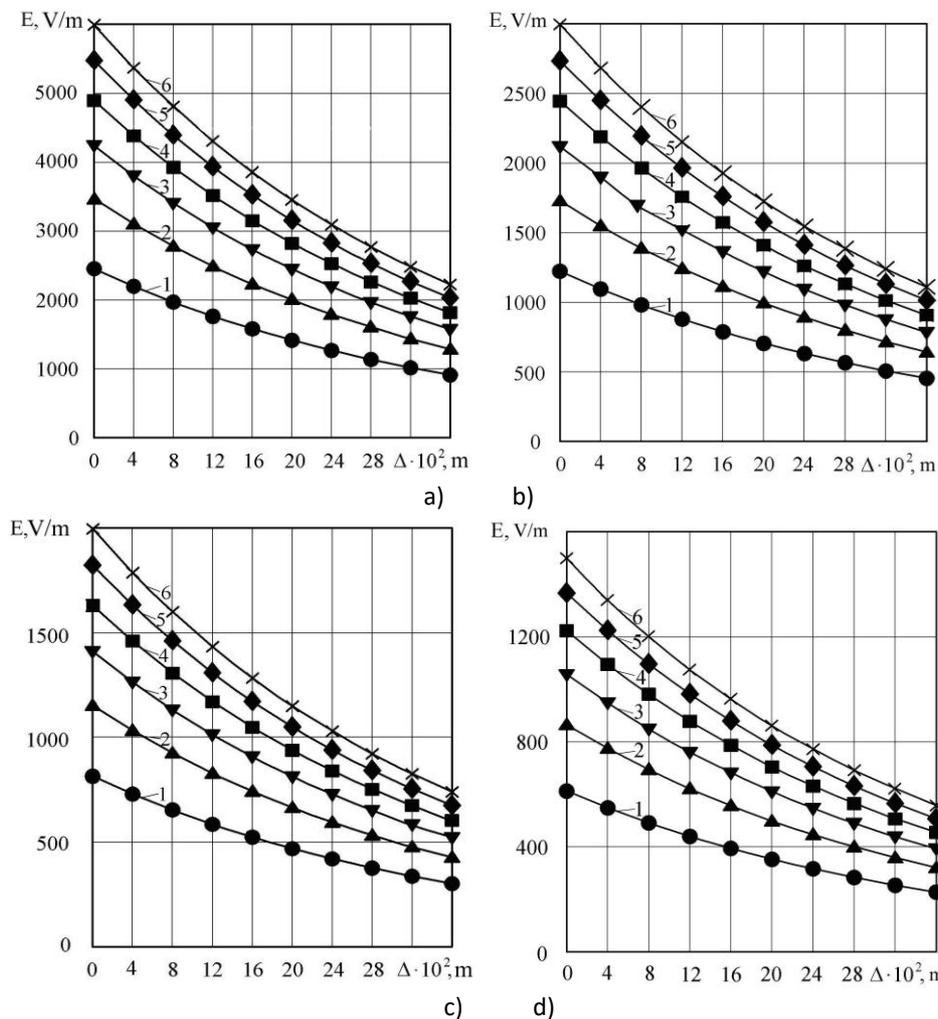
Fig. 2. Magnitude of strength of electromagnetic field depending on the thickness of the layer ( $\Delta$ ) and microwave power ( $P$ ) for mixture of finely-chopped greenery of spicy vegetables: 1 – 500 W; 2 – 1000 W; 3 – 1500 W; 4 – 2000 W; 5 – 2500 W; 6 – 3000 W, for surface area of a product: a – 200 cm<sup>2</sup>; b – 800 cm<sup>2</sup>; c – 1800 cm<sup>2</sup>; d – 3200 cm<sup>2</sup>
