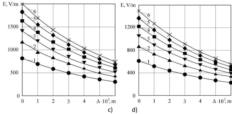
Fig. 1. Magnitude of strength of electromagnetic field depending on the thickness of the layer ( $\Delta$ ) and microwave power ( $P$ ) for mixture of finely-chopped roots of spicy vegetables: 1 – 500 W; 2 – 1000 W; 3 – 1500 W; 4 – 2000 W; 5 – 2500 W; 6 – 3000 W, for surface area of a product: a – 50 cm<sup>2</sup>; b – 200 cm<sup>2</sup>; c – 450 cm<sup>2</sup>; d – 800 cm<sup>2</sup>.
