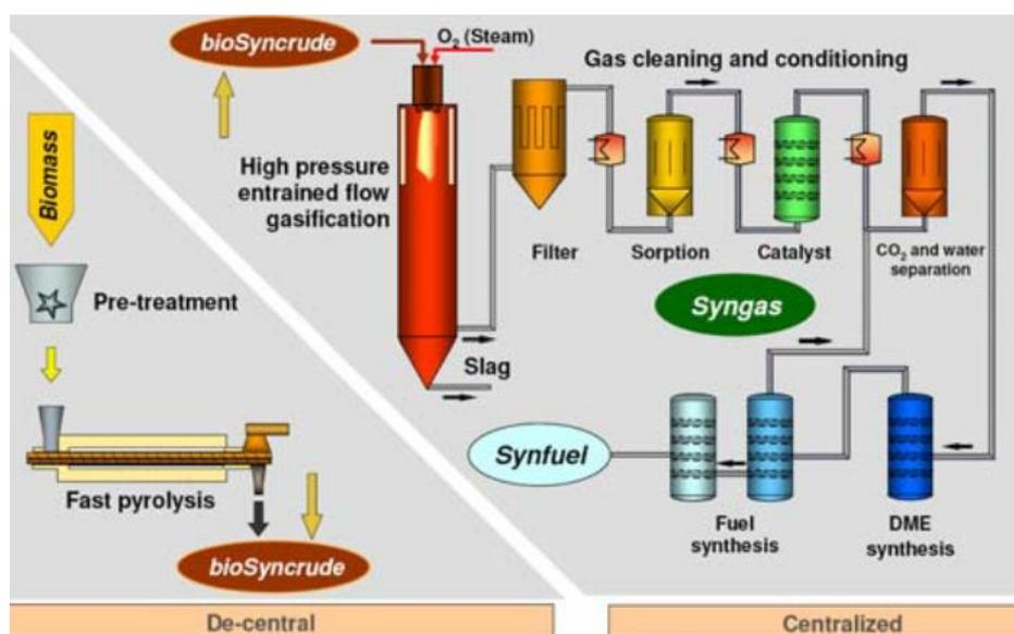
Fig. 8. The bioliq plant – process diagram. Source: [9]
