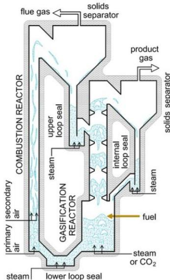
Fig. 4. Gasification system G-voution developed at VUT. Source: [6]
