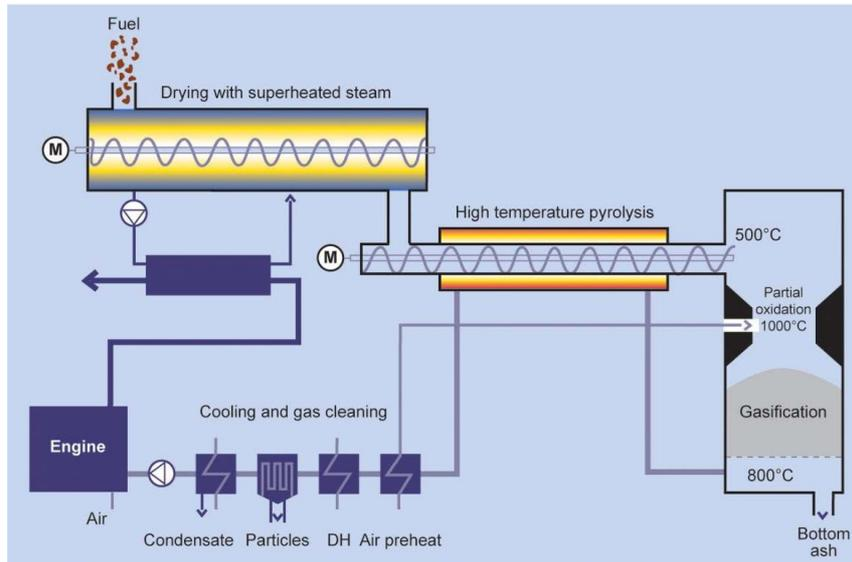
Fig. 6. VIKING gasification system developed at DTU. Source [7]
