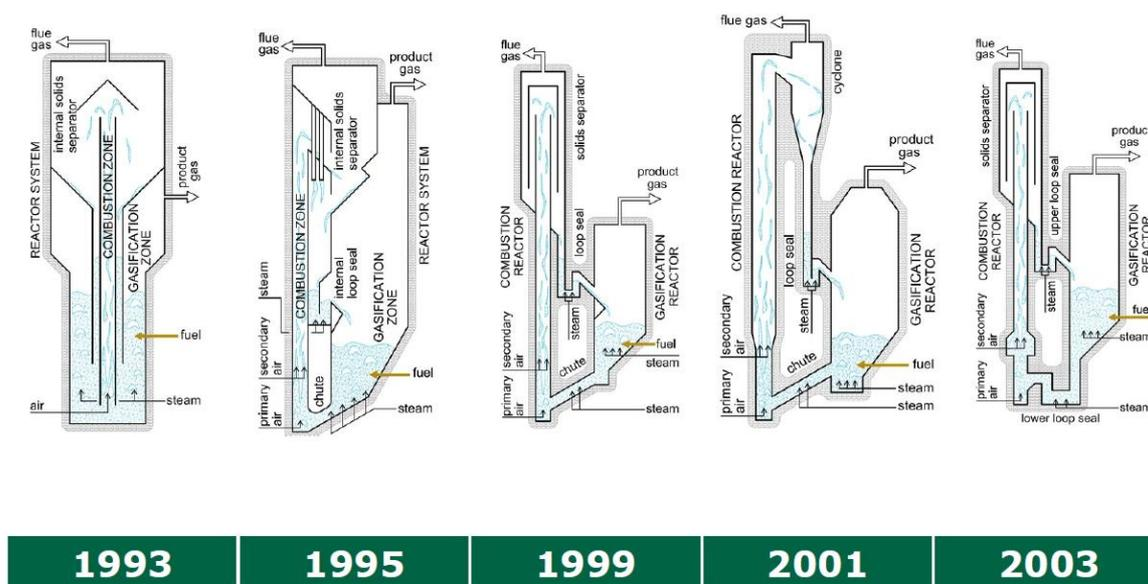
Fig. 3. Research at VUT - development of dual fluidized bed. *Source: [6]*
