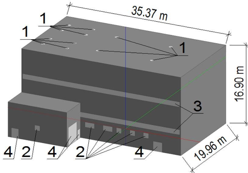
Fig. 1. Building geometrical model, where: 1 – exhaust roof fan, 2 – air intake, 3 – window, 4 - door
