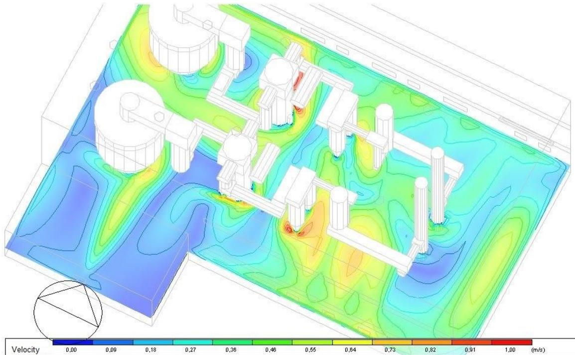
Fig. 4. Air velocity distribution on the level of + 1.70 m
