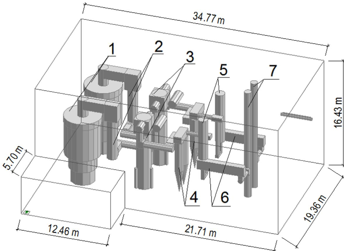
Fig. 2. Room geometrical model, where: 1 – furnace, 2 recuperator, 3 – boiler, 4 – multicyclone, 5 – steam cooling device, 6 – bag filter, 7 – chimney
