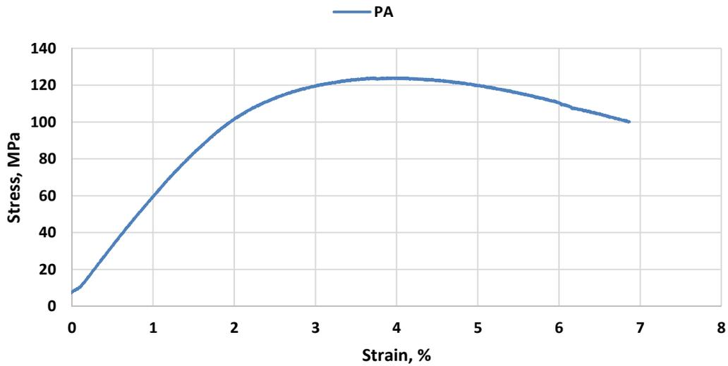
Fig. 5. Results of bending strength investigations of polyamide
