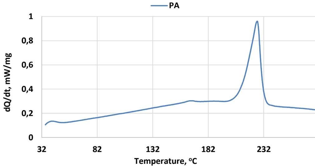
Fig. 1. Thermogram of polyamide.
