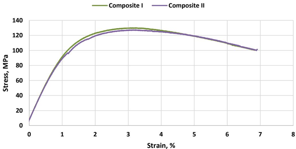
Fig. 6. Results of tensile bending investigations of polyamide of composites
