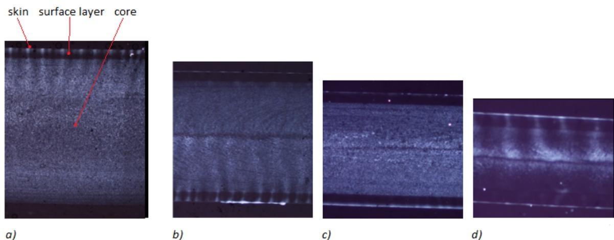
Fig. 9. The morphology of injection molded parts from polypropylene at different wall thicknesses: a) 1 mm, b) 2 mm, c) 3 mm, d) 4 mm
