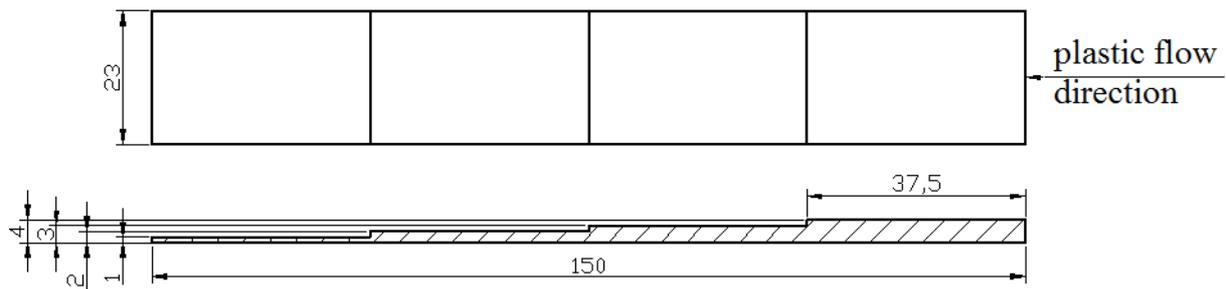
Fig. 3. Shape and dimensions of test sample
