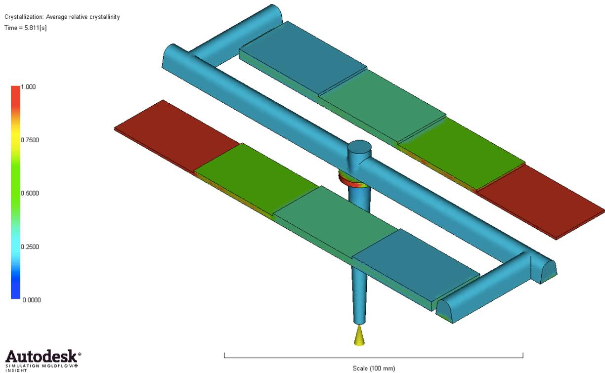
Fig. 6. Average relative crystallinity of molded part with various thicknesses from HDPE
